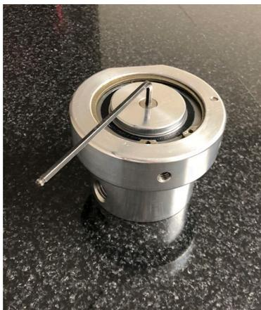
Reset center cover plate to the middle of the now reversed Drive Sentry and secure in place by tightening the flat head screw with .1875" Allen Wrench.
