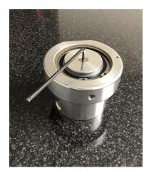
Reset center cover plate to the middle of the now reversed Drive Sentry and secure in place by tightening the flat head screw with .1875" Allen Wrench.
