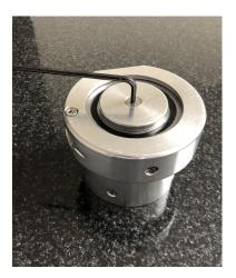
Use .1875" Allen Wrench to remove the flat head screw at center of bottom plate on the bottom of Drive Sentry.
