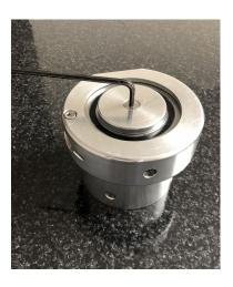
Use .1875" Allen Wrench to remove the flat head screw at center of bottom plate on the bottom of Drive Sentry.
